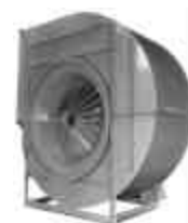
Arrangement 1, SWSI, Class III fan with rigidly braced housing, split for ease of wheel removal and inlet vane control.
